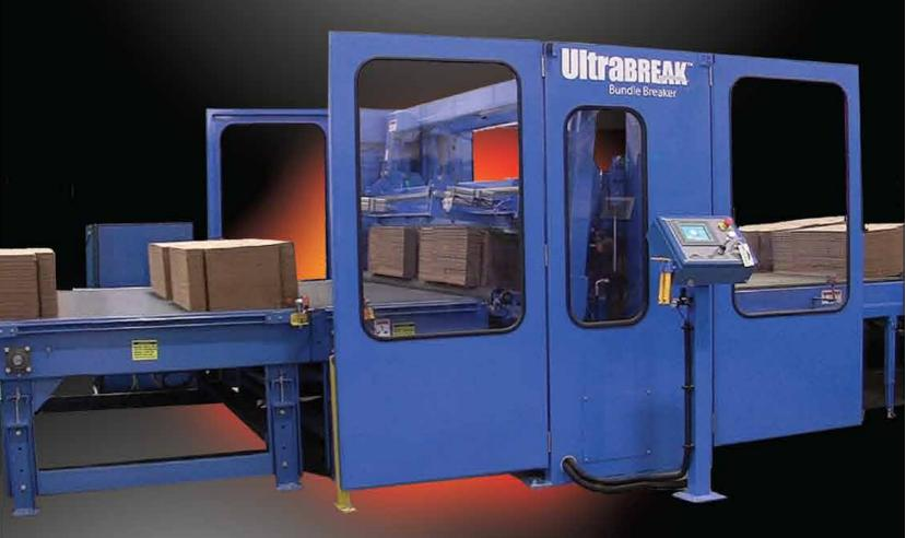
Faster Cycle Times are a result of improved controls with optimized position sensing to reduce overall platen travel during the break cycle.
