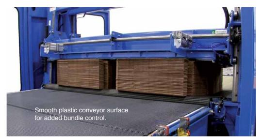
**Up-Break Machine Motion** has been specially optimized to reduce platen travel during the break cycle, resulting in faster cycle times. The Up-Break motion
