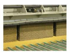
Segmented floating platen design allows true multipleacross breaking performance for bundles with slightly unequal heights.
