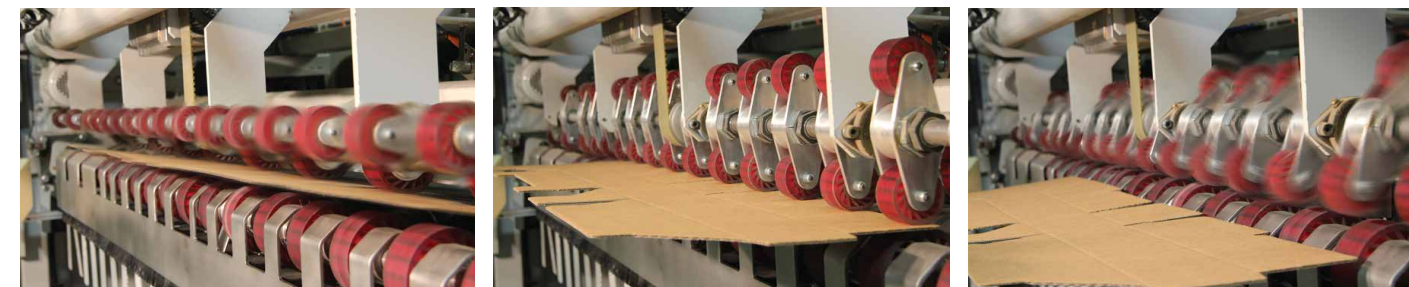
1. Blanks enter the TEDD at machine speed or higher
